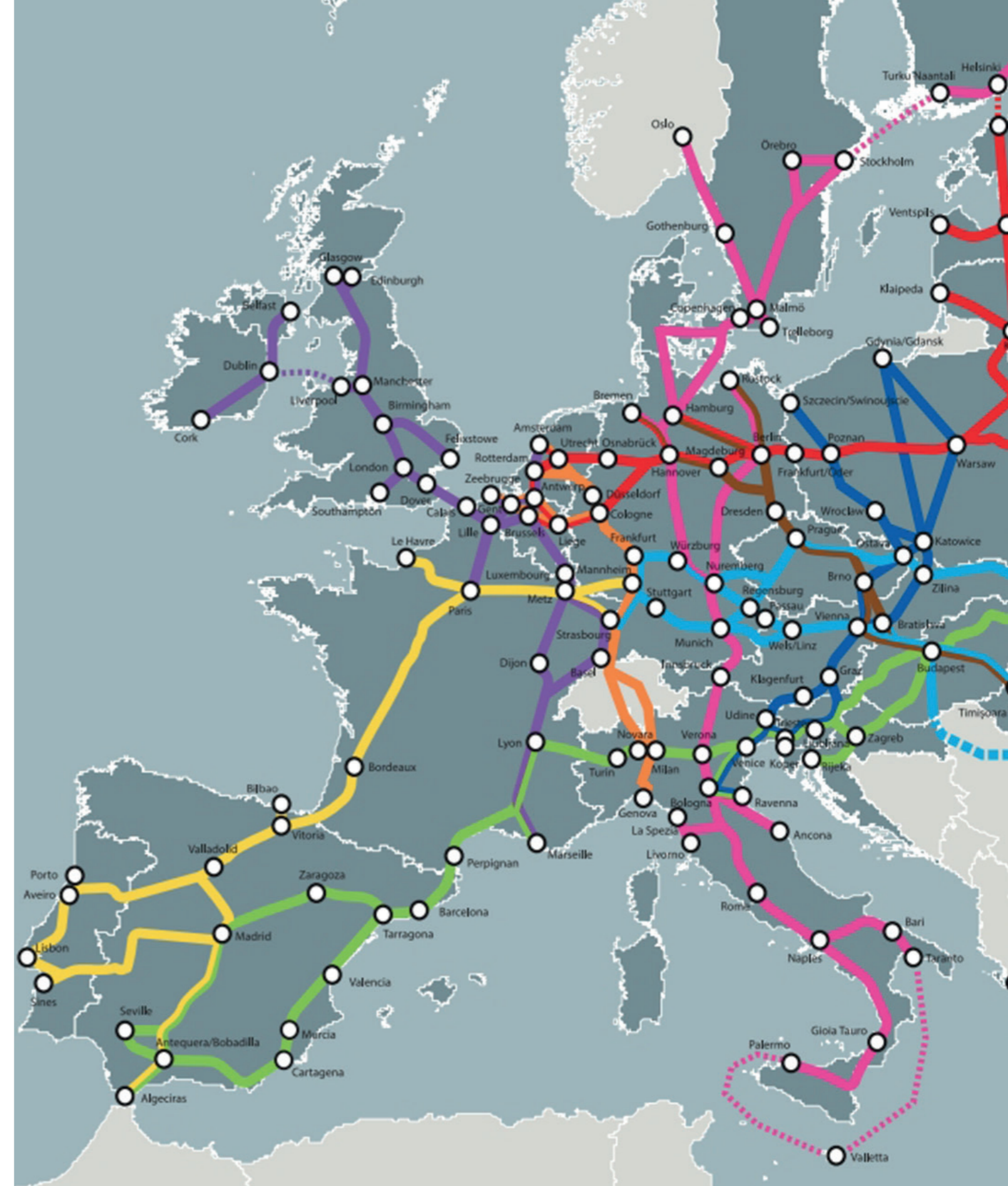
Ten-T consists of a core network with nine corridors that link together key hubs in Europe. A common signalling system and rail freight corridors should be completed by 2030. The ScanMed corridor (pink) links the Nordic capital cities (Oslo, Copenhagen, Stockholm, Helsinki) with the Mediterranean (major cities and coastal ports in Italy, Sicily, Malta). Source: The EU Commission
